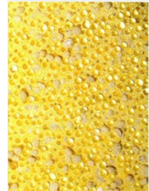
Exhibit 20: Closeup of Recess Triple Drop pavement marking, with glass beads and ceramic elements
